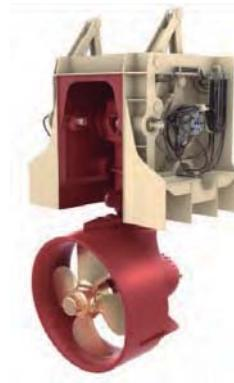
Units are supplied complete with a small hull module carrying all the lifting, locking, steering and transmission systems. This weld-in module has a small footprint and can be trimmed by the yard to suit the installation. The yard provides the rest of the garage so it can be designed to match the hull lines.
