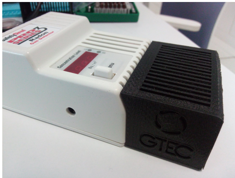
Figure 6. Radon sensor with the 3D-printed black box that contains the added electronics.
