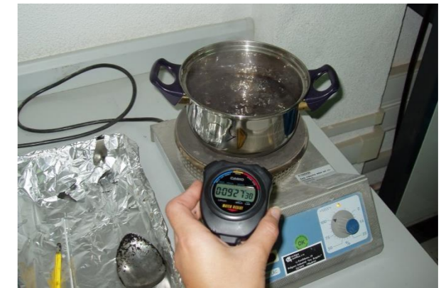
Loose mixture in boiling water for 10 minutes
