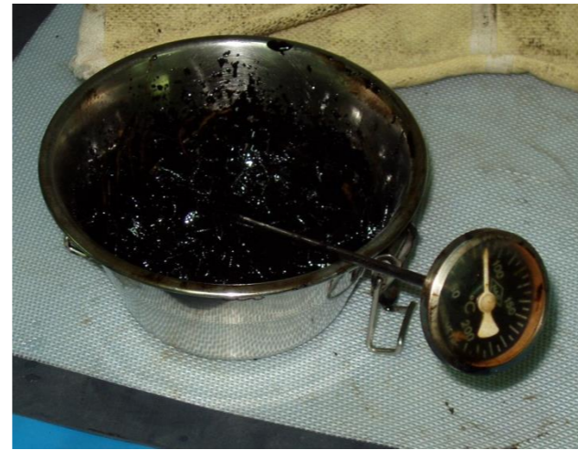
The loose mixture temperature must be between 85 °C and the boiling temperature of the water
