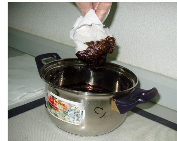
Free bitumen is skimmed of from the water surface
