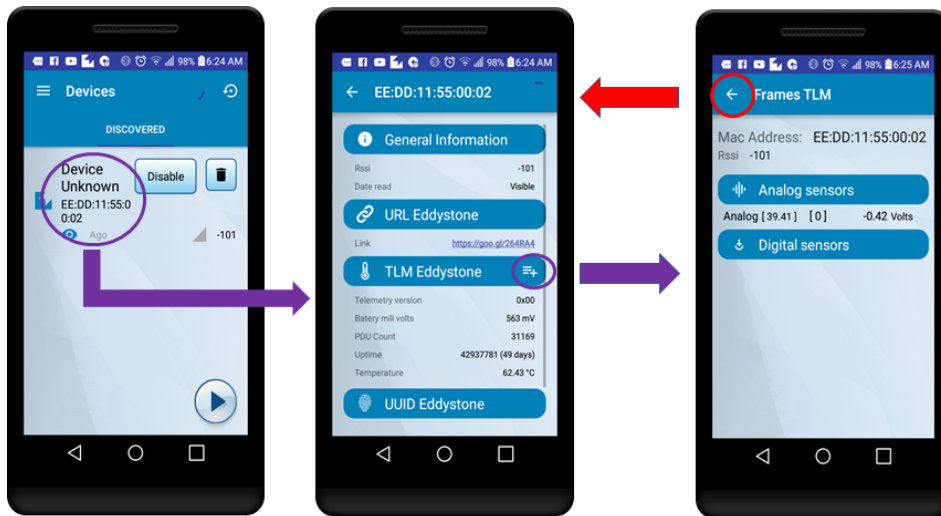
Figure 20. Accessing the embedded information through the Android app.
