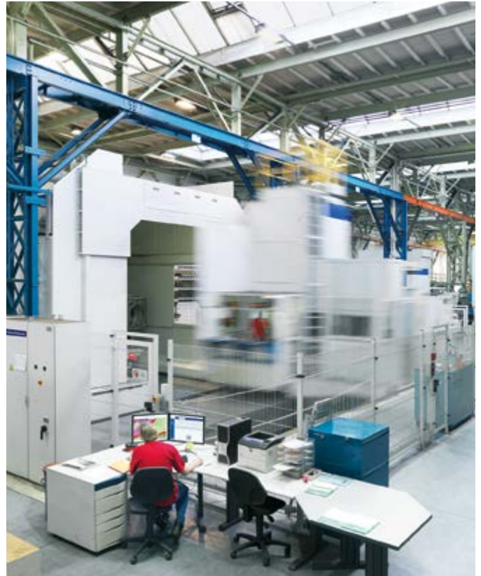
Dörries Scharmann, Heavyspeed CNC Milling Machine Centric table load: 40'000 kg, spindle stroke: 1'000 mm
