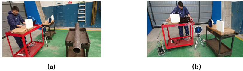
Figure 9. Measurements with passive UHF reader with four antennas. (a) Linear array; (b) L-shaped array.
