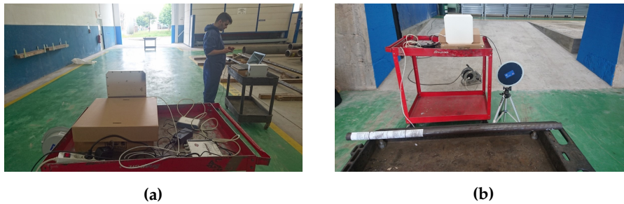
Figure 7. Measurements with passive UHF reader with two antennas. (a) At 17 m; (b) At 2 m.
