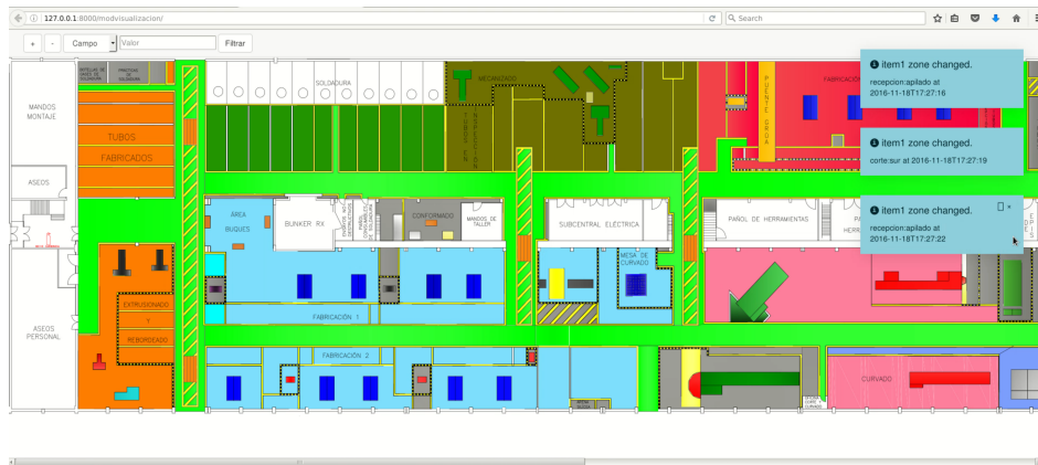
Figure 25. Notifications shown on the right upper part when a pipe crosses from one area to another.
