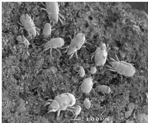
Figure 5. SEM photograph of mites on perlite granules in biofilters (Wageningen University; research project of TNO Environment, Energy and Process Innovation and Bioway).
