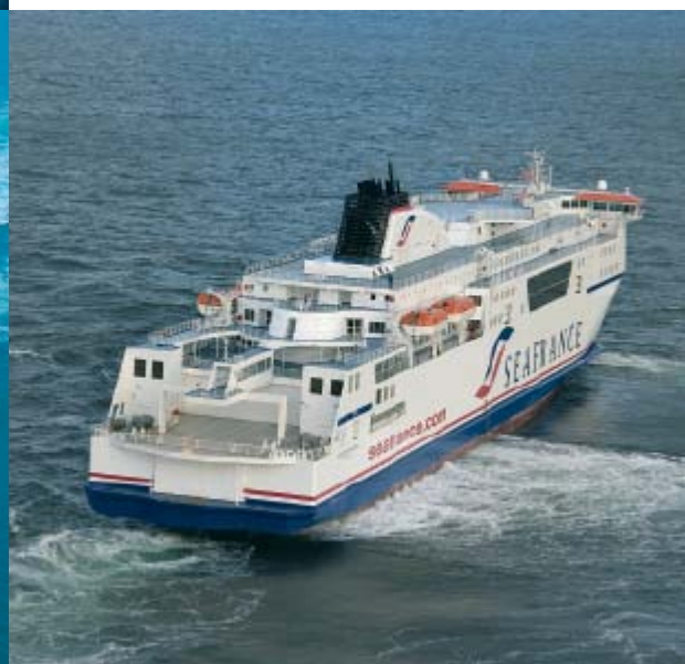
The passenger RoRo vessel Seafrance Rodin is equipped with four LIPS CT225 transverse thrusters.
