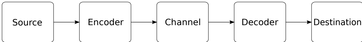
Figure 1.2: Block diagram of a JSCC system.
