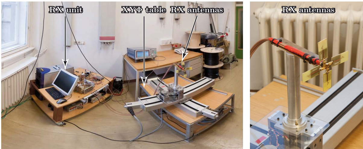
Figure 8.4: Photograph of the scenario at the RX side. The testbed RX is shown as well as the four printed monopole RX antennas [167, 168] mounted on the XY\Phi positioning table.
