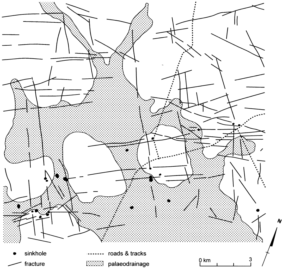
Fig. 8. (c) Plan of part of Sturt Plateau, northern Australia, developed in laterite over Cretaceous strata, showing the relationship of dolines to fractures and palaeochannels (drawn from air photographs).
