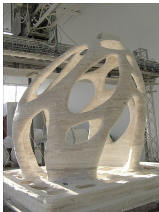
Fig 4. Radiolaria Pavilion, D Shape System, Enrico Dini, 2008
