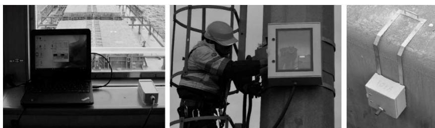
Figure 2. Left: IMU (Inertial measurement unit), Center: Photogrammetric techniques, Right: Laser distance sensor.
