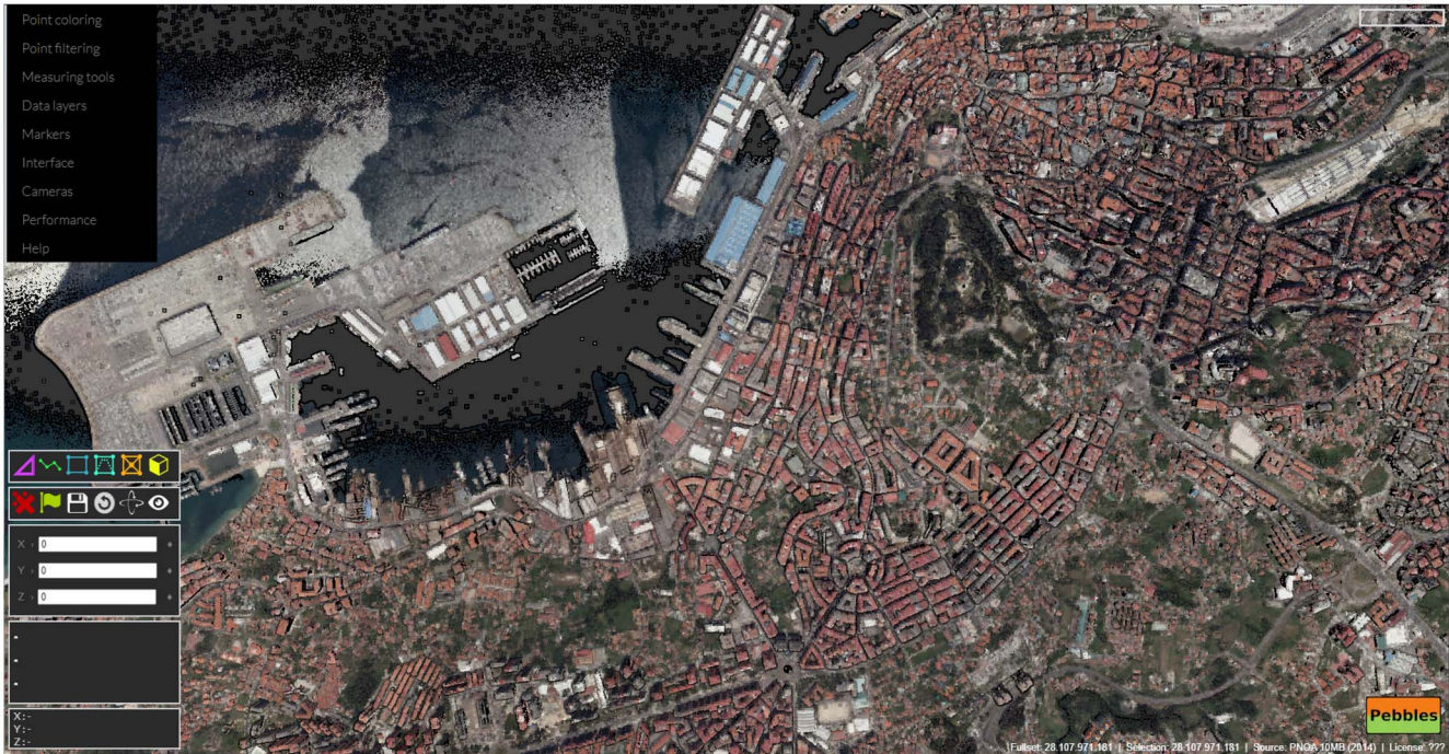
FIGURE 9. Part of PNOA dataset using 5 MB as CS being rendered with 8 million points using color data from satellite.
