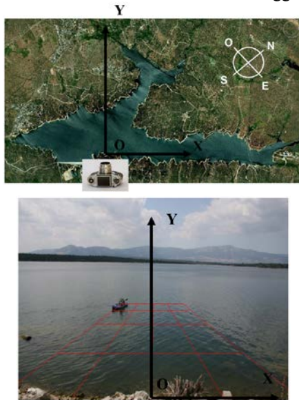
Figure 2 (a) Camera placed on the shore of the reservoir; (b) An image of the 3D scene as it is seen by the camera.
