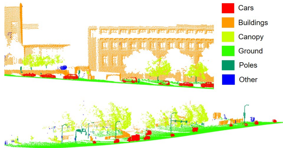
Figure 7. Oakland MLS point cloud. The classes to be extracted have been represented in different colors.
