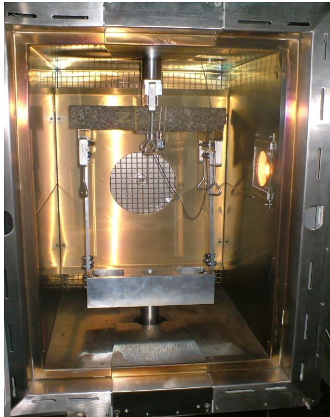
FIG. 1. Bending fatigue test
