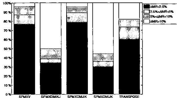
Figure 4.11: Percentage of the number of experiments in which the \Delta_{MR} is below 2.5%, between 2.5% and 5%, between 5% and 10%, or larger than 10% when real matrices with a non-uniform distribution of the entries are used.
