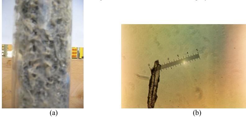
Figure 2. (a) Developed biofilm on the stainless steel packing, (b) Micro-photograph of detached biofilm.
